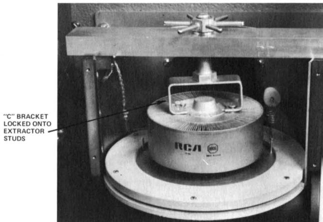
Figure 7 – RCA Tube Type 8806 Ready to be Removed From Cavity Y1116A
