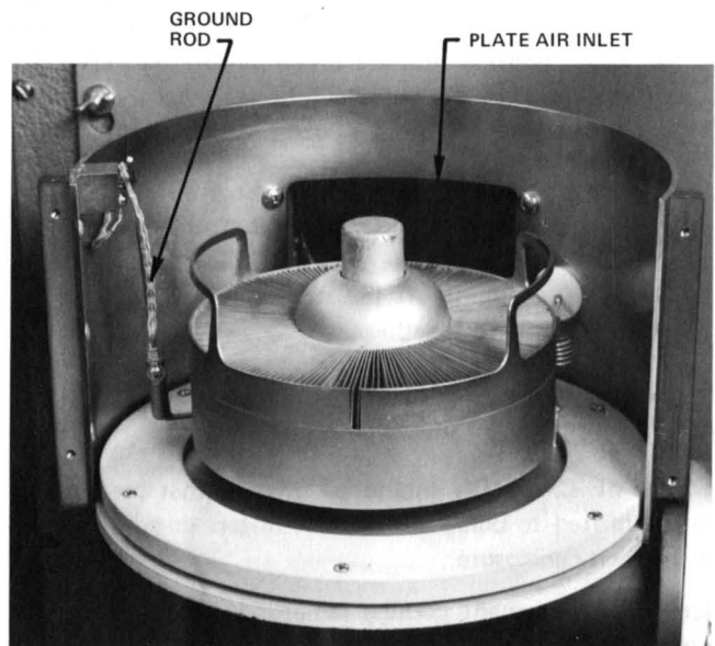
Figure 1 — RCA Tube Type 8807 Installed in Y1116B Cavity
